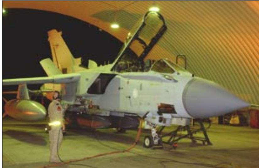
**A Tornado GR4, armed with two Storm Shadow stand-off missiles, is prepared for a sortie**
