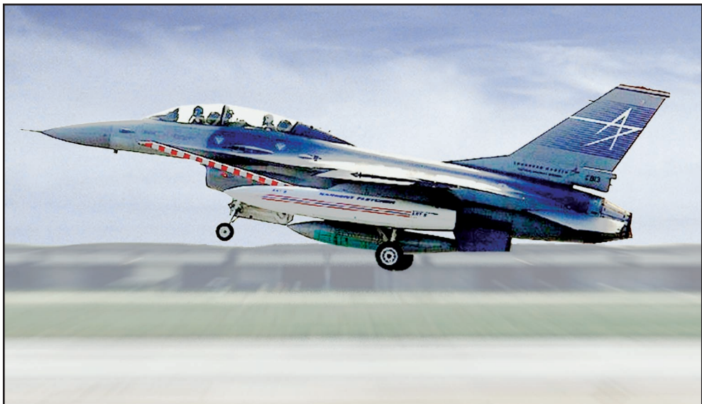
Sargent Fletcher's 27-370 ART/S ® Pod mounted on Lockheed Martin's F-16, station 4, during take-off.
